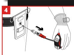
Attach the holster to your work belt by the sliding belt through the rear straps of the Tape Measure Latch Holster.
