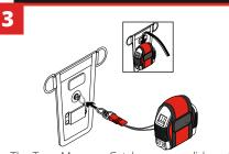
The Tape Measure Catch can now slide onto the Tape Measure Latch.
