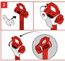
Assemble the two parts together. Loop the "Wings" over each side.
