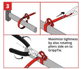
Wrap the GrippTie around the tool, the logo and text should be visible on the outside. Feed the strap through and pull the tag end until the GrippTie is firmly in contact with the tool, this will require a pair of pliers.
