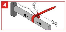
Check that the GrippTie is sufficiently tightened. Pull by hand in each direction. It should not move. Then snip off the tag end. Take care not to make any sharp edges.
