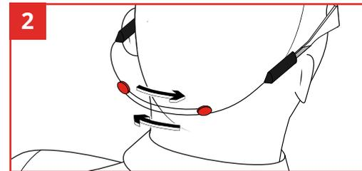
Place eyewear and Safety Glasses Tether on head. Adjust the Safety Glasses Tether by sliding the two red central pieces to opposite sides.
