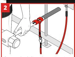
Connect to handrail or tool connection point.
