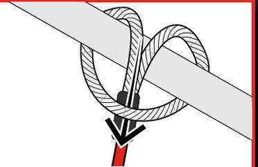
Feed the carabiner end of the tether through the loop and pull tightly to create a secure connection.
