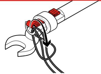
To attach using the loop end, pass the loop through a connection point.
