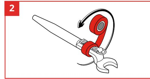
Wrap the tape around the tool 10x while stretching the tape to activate the self-vulcanizing feature, creating a secure connection. Ensure raised 'catch' is not covered by the tape. Pull on Tool Catch with force to test application.
