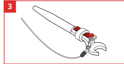
Your Tool Catch is now ready to be connected with a suitable GRIPPS® tether via the D-Ring.
