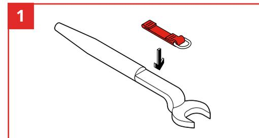
Place Tool Catch with metal ring facing away from the tools center of gravity, white tag facing up.
