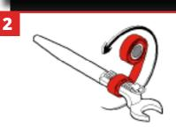
Wrap GRIPPS® V-Gripp Tape around the tool 10 x while stretching the tape to activate the self-vulcanising feature, creating a secure connection. Ensure the raised catch is not covered by the tape. Pull on Tool Catch with force to test application.
