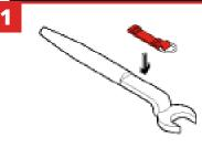
Place Tool Catch with D-ring facing away from the tool's center of gravity.
