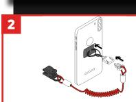
Secure E-Tether to E-Catch by first feeding loop through the connector point, then feed the E-Tether back through the loop to create a choke.
