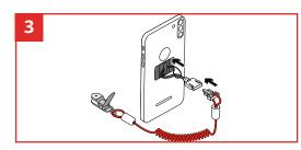
Secure E-Tether to E-Catch by first feeding loop through the connector point, then feed the E-Tether back through the loop to create a choke.
