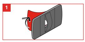
Peel cover from one side of the adhesive pad and attach to the E-Catch. Peel cover from other side and attach to a non-porous location on the device.
