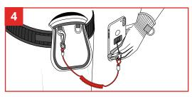
Press side-release buttons to hot-swap between different electronic devices. Ensure attachment dock 'clicks' back into place.
