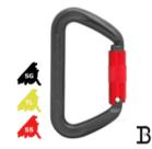
KH218 Aluminium Wizard Weight 113g (40z) Gate Opening 29mm (1 1/8") MBS 40kN (8992lbf) Height 128mm (5") Width 73mm (2 7/8")
