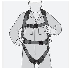
Fitted harness should be snug and firmly fitted, particularly the leg straps
