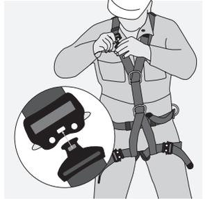
Repeat for right shoulder strap and connect the buckle. Ensure green spot can be seen in the receiver window
