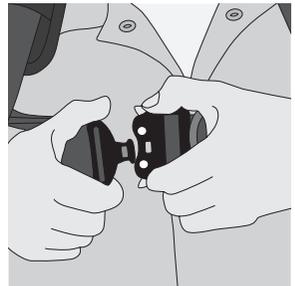
To release, push the two side tabs simultaneously and separate the buckles
