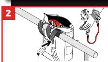
To secure to a rail, wrap the velcro mounting straps all the way around the rail and feed back through the metal brackets. Adhere velcro strap.
