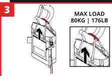
To lift, zip the lid closed to secure contents. Ensure all tools are tethered to D-Rings. Attach lifting hook to both lifting straps.
