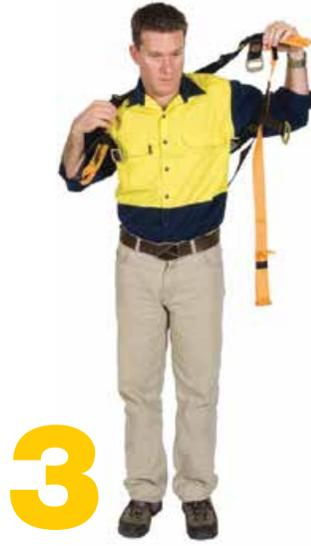
Rotate harness and insert elbow into arm loop and then place arm through the other shoulder loop and let harness fall onto the shoulders. Ensure that the harness is fitted correctly without any webbing twists over the shoulders.
