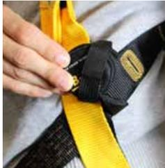
2. Choke unit onto strap by passing body through case loop.
