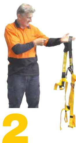
Hold harness to your left side by left shoulder strap and right shoulder buckle and slip on shoulders sideways holding large part of buckle in right hand.
