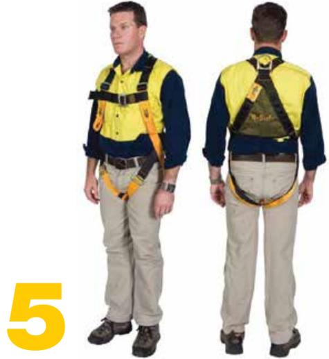
Adjust shoulder straps first to ensure that the rear dorsal D is located between the shoulder blades in the centre of the back. Then adjust chest and leg straps to a firm fit, and slide webbing keepers along to hold free webbing in place.
