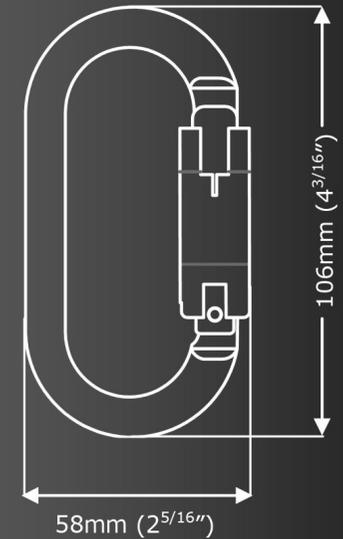
ISC Performance Karabiners are forged for best build quality. The Barrels have been designed with a square cut notch to limit debris build up.
