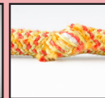
Serious sheath damage
