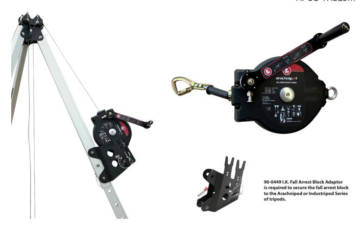
The APOD-FAB25 is a Type 3 Rescue Recovery Block which arrests a fall and also enables simple retrieval of the victim. With 25 metres of galvanised steel wire, the fall arrest block is compatible with the Ferno Arachnipod system, Industripod and Industripod+ tripods when used in conjunction with the I.K. Fall Arrest Block Adaptor.
