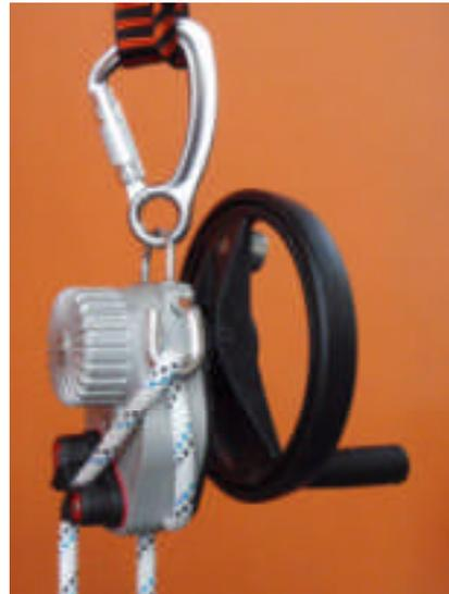
The handwheel can be rotated to elevate the accident victim till he/she can either be lifted to a secure base or the securing lanyard of the person to be rescued can be detached. When doing so, the slack rope between the turning device and the cam cleat is pulled downward and tightened over and over again. This helps in minimising the distance over which the person to be rescued may slip in case the handwheel is inadvertently released.
