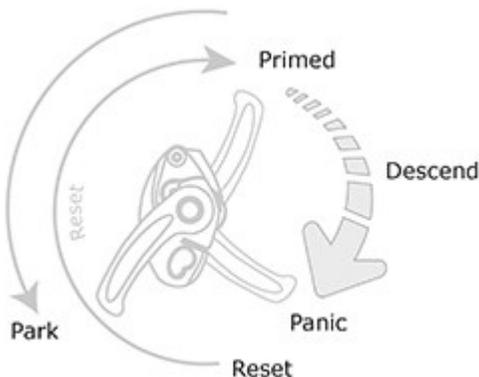
The D5 features a progressive cam action, which offers precise control during low or high speeds. The cam is made from high grade, solid Stainless Steel, for maximum durability, even in harsh environments, such as Geotech work.
