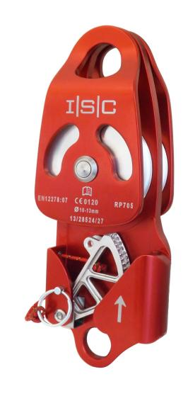
To assist in controlling the lower/release, the one-way bearings (when roped correctly) will not turn, which means that they then act as a static bollard thereby giving the operator greater control.
