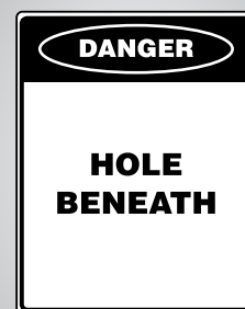
FIGURE 5 Example of the type of danger sign to be affixed to the hole cover.
