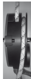
(Q) Run rope downwards and control abseiling operation manually. If necessary, secure the rope in the rope clamp.
