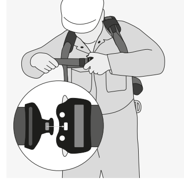
Connect chest buckle, ensuring that green spot is seen in the receiver window. Tighten strap.
