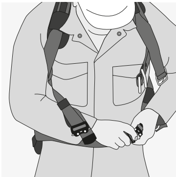
If a waist belt is fitted, connect and tighten
