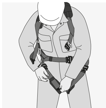
Tighten straps and retain free webbing within the elastic webbing
