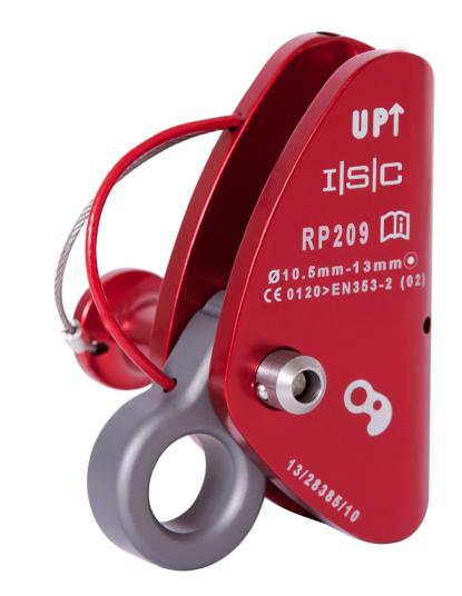
ISC Ropegrabs have a non-aggressive cam-face design which helps prevent rope wear.
