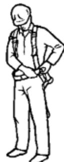
7. Pass both leg straps between your legs making sure there are no twists in the straps. **NOTE: Leg strap quick connect buckles are black coloured.** Connect the left leg strap's Quick Connect buckle to the left leg link, and the right leg strap to the right leg link. Adjust both for a comfortable fit.
