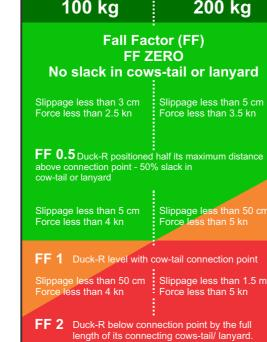
The Duck-R has successfully been tested by the manufacture to with loads of 200kg. This testing is designed to replicate rescue techniques and requirements with limited lanyard lengths and limited Fall Factors. The testing produced provided consistent performance.
