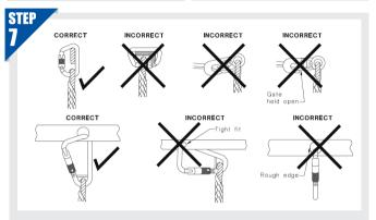
PUT ROPE THROUGH KARABINER AND ENSURE KARABINER HAS BEEN FITTED CORRECTLY
