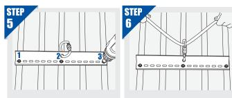
FIX THE TETHER PLATE TO THE CENTRE LINE OF THE ROOF BATTEN OR PURLIN WITH A MINIMUM OF 3 SCREWS TO ACHIEVE 15 KN FIT KARABINER TO LOADING EYE WITH LOCKING DEVICE FACING UPWARD
