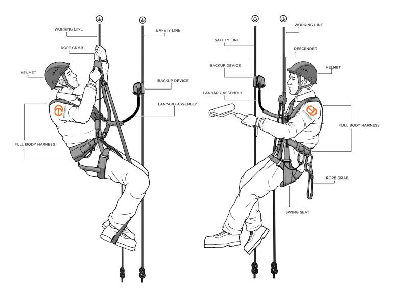
The list covers a select range of Rope Access equipment that is commonly used in Australia by rope access technicians. There is a large range of equipment not listed that is suitable for rope access. Care must be taken when selecting rope access that it is fit for purpose and meets relevant standards. Training to ensure that the user is competent in the correct use of this equipment must also be undertaken.
