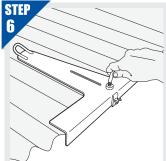
ENSURE L BOLT IS TIGHTENED ONTO ROOFING IRON TO CLAMP ANCHOR TO ROOFING IRON.
