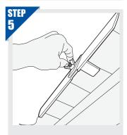
ENSURE WING NUT IS TIGHTENED TO SECURE BOTTOM TAB AS SHOWN
