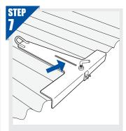
SCREW IN A ROOF SCREW
